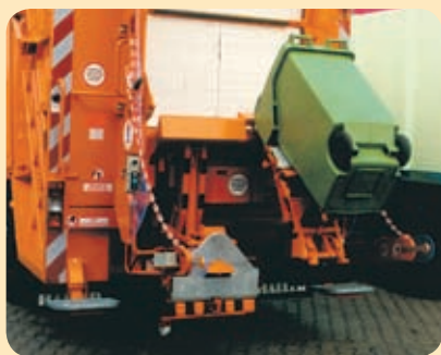
rear loader with combined comb/diamond-lifter
