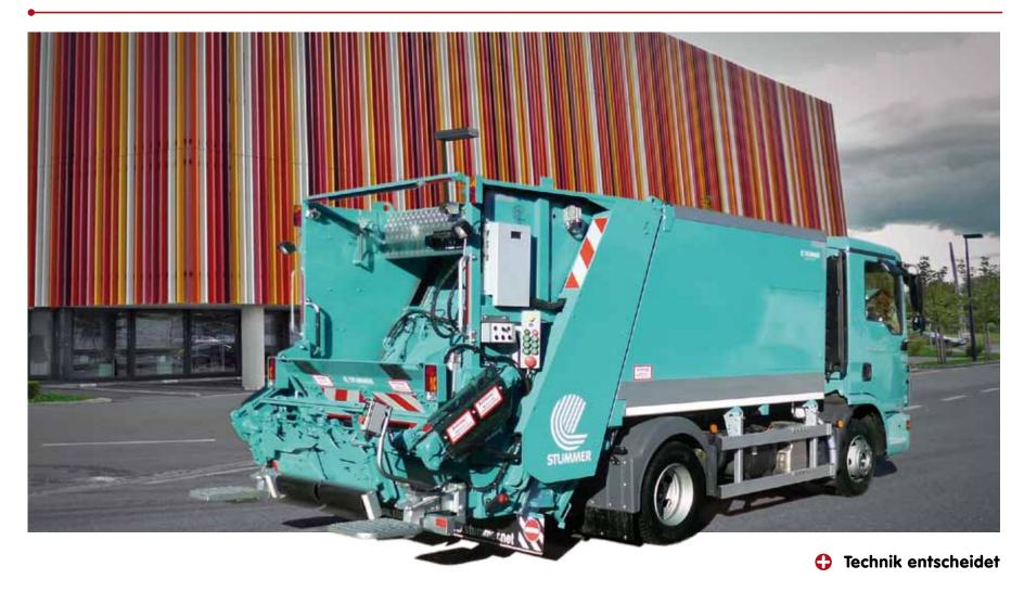
The high performance vehicle for narrow streets. The compact dimensions of this vehicle are ideal for inner city areas with narrow accesses and low entrances. The Mini is the smallest regular RCV that fulfils all requirements and, due to its robust structure and high payload, it is better in some cases than larger vehicles. The integrated lifter allows the emptying of bins up to 1.1 cbm.
