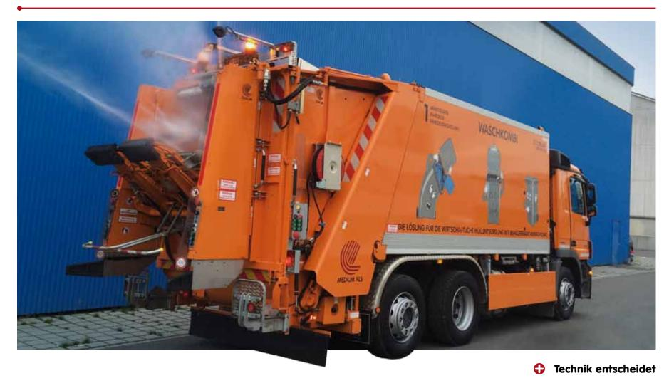
The Stummer bin washing device combines the disposal of refuse with the cleaning of bins in one operation with one vehicle and one team. Thus the requirements of households to have hygienic containers can be met in a very economic way.
